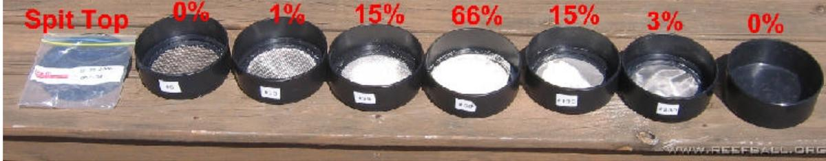
Sometimes you will want to know more about the composition of the sand. Take a small sample and view with a magnifying lens. Sorry, this is slow work. It can be useful to understand the type of sediment stressing the corals. Generally terrestrial-based (round sand grains) are more stressful to corals than irregular shaped coral or shell sands.
