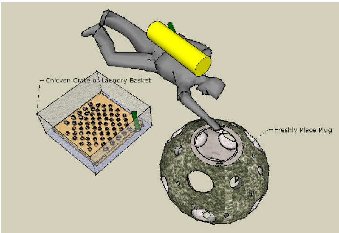
Figure G34: Schematic of diver planting coral plugs from a Coral Planting Tray onto a Reef Ball. The diver can use the tray to store supplies such as a wire brush, or extra epoxy putty.
