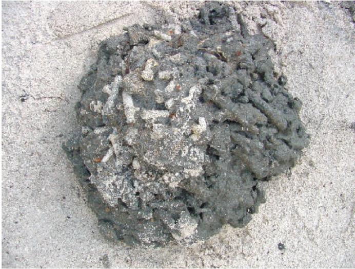
*Figure 13: Reef Forms are large blobs of concrete cast into a mold made of sand and affixed with coral adapter plugs. Reef Forms*
