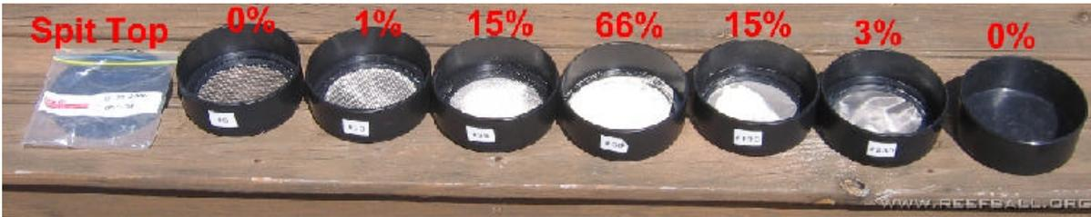
Figure 8: Results of a sediment grain size analysis. A sample of sand is passed through stacked sieves with decreasing sized mesh. The proportion of the sample retained in each sieve can be used to approximate the distribution of grain sizes in the sediment at the site.
