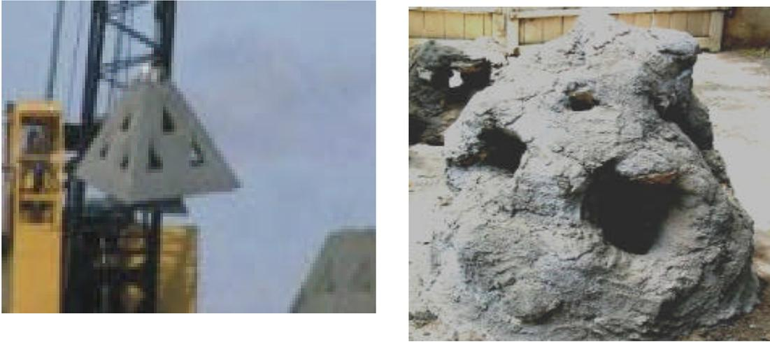
*Figure 16: Concrete modules designed primarily for ‘fish only’ projects. Left: Artificial Reefs 1 Fish Haven™ Modules. Right: Hand made ‘Fish Houses’. Modules of these types are not recommended for coral rehabilitation techniques discussed in this manual because they utilize support frames made from metal, which can reduce the long term durability and stability of the module.*
