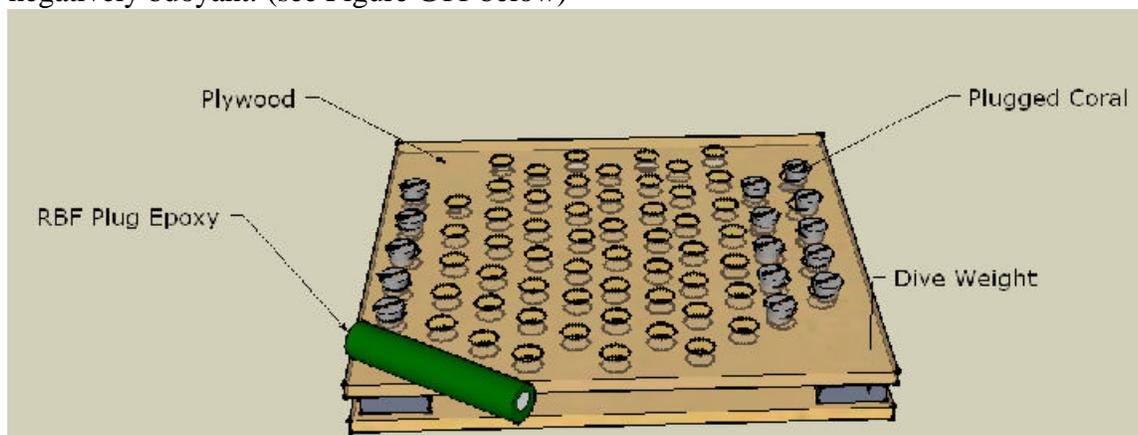
Figure G18: Diagram of Coral Curing and Planting Tray (available in Sketch Up™). Coral Plugs fit into the holes drilled in the top board, which can be made from plywood or, if available, more water resistant materials such as resin or plastic.
