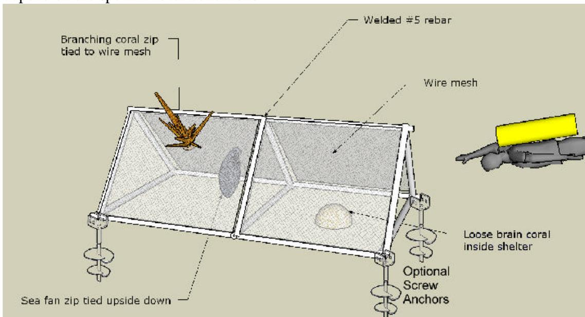
*Figure 2: A temporary disaster nursery constructed from wire mesh attached to a tetrahedral frame made from welded steel. Imperiled corals would be attached to the wire mesh with plastic cable ties or thin wire to protect them from damage by waves or sedimentation until a permanent solution can be implemented. If necessary, “disaster nurseries” can be anchored with screw anchors*
