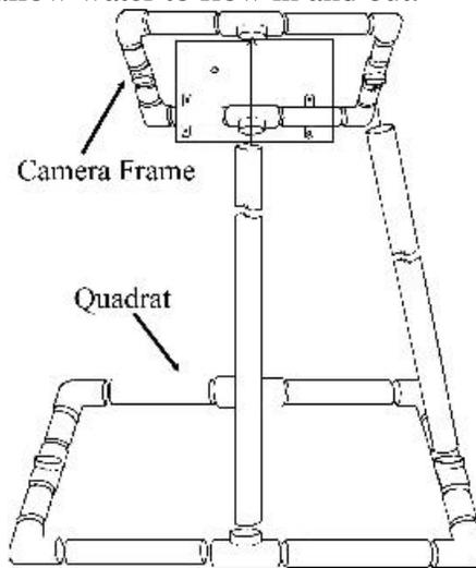
Figure G30: Camera monitoring frame or quadrat framer. This device is built so that most standard underwater digital cameras can screw into the plate in the center of the camera frame, and will take a picture downwards towards the quadrat. The quadrat allows the photo to be standardized for length.
