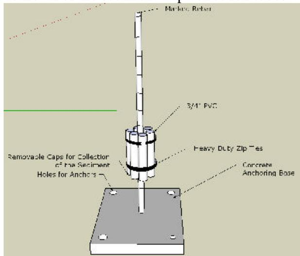
Figure 9: Construction of a basic sediment trap to estimate sedimentation rates at a project site. Sediment accumulates in the PVC tubes, and can be retrieved and measured (by weight or volume) by removing the caps at the bottom of the PVC tubes and collecting the sediment within. Note: This method only provides a relative estimate of the amount of sediment at a specific depth, and not an exact value because it measures the vertical settling of sediment, and not horizontal transport.
