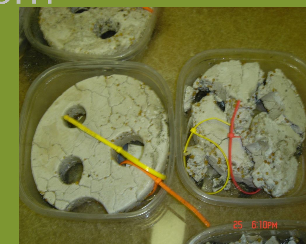
Figure 4: Fert -Discs undergoing laboratory tests. Note structural integrity of cement fortified (left) vs. unfortified (right) plaster
