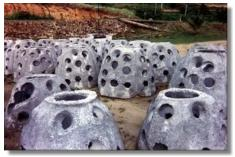
Reef Ball<sup>TM</sup> project. Hollow concrete domes are produced to eventually be towed and placed on the ocean floor to enhance coral and fish habitat - Fajardo, Puerto Rico.
