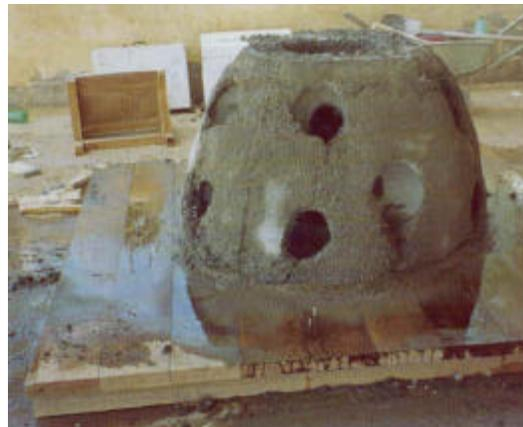
*Left, tile concrete mixture is poured into a mould, the little side holes contain file balloons that form the desired tunnels and are later deflated. Above, fresh water is sprayed to roughen tile surface soon after the concrete mixture is released from the mould.*
