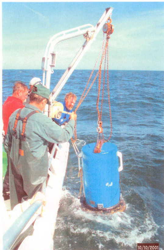
Figure 8. Retrieving an experimental reef habitat unit encapsulated in a plastic drum.
