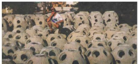
Larry Beggs, vice president of the Reef Ball Development Group, crouches on a concrete artificial reef, similar to ones being installed in Tampa Bay. The reefs are part of a project designed to attract oysters and other marine life, which in turn should help clear up the effects of stormwater runoff.
