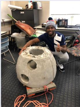
Figure 1: Each Mini-Bay Ball RBM weighs 90kg and provides 2.9m<sup>2</sup> of surface area and was constructed using materials and guidelines provided by the Reef Ball Foundation.
