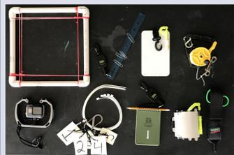
Figure 7: Pictured above is all the materials needed for Method 2. This includes: 1 Quadrat, 1 Ruler with 4 paper clips attached, 1 Write in the rain booklet, 1 GoPro in a waterproof casing, 5 zip ties with numbers attached, 1 retractable spool to attach diving flag to, 1 pair of shears, and 2 dive slates.
