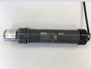
Figure 9: HOBO MX2501 pH and Temperature logger by Onset was placed on the RBM on 3/21/19 and picked up on 3/28/19. The logger collected data in 15 minute intervals for one week.
