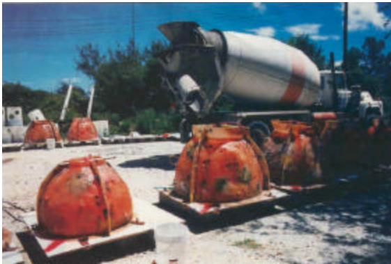
Reef Ball molds and demolding of a Reef Ball reveals its Swiss-cheese-like holes and internal inflated balloon.
