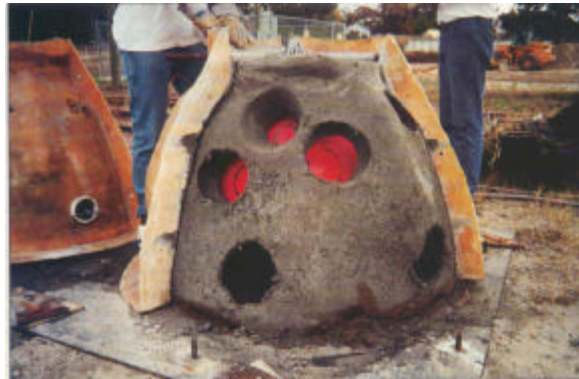
Reef Ball molds and demolding of a Reef Ball reveals its Swiss-cheese-like holes and internal inflated balloon.
