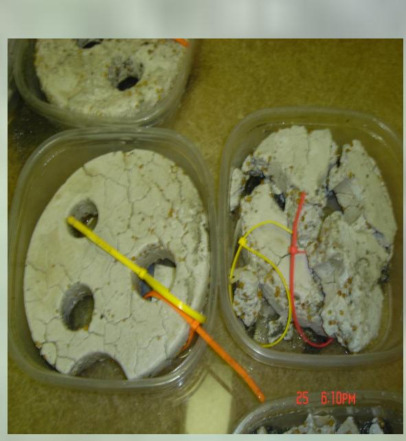
Figure 10: Discs made from 100% PoP (right) vs. an 80/10/10 mixture of plaster/sand/portland (left) Discs shown are approximately one month old.
