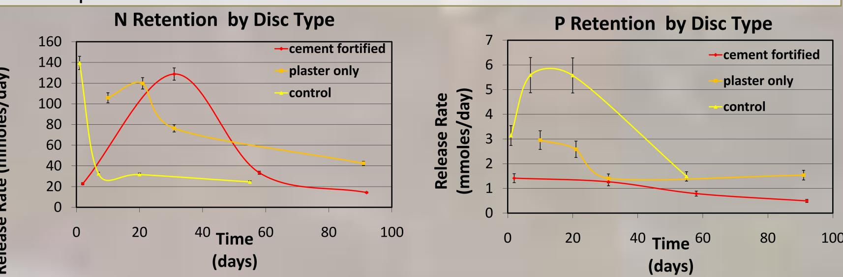
Figures 7 &8: Release rate in millimoles of N (left) and P (right) per day for plaster, cement fortified plaster, and control (no disc, just fertilizer) treatments. 50 grams of fertilizer were used per treatment. Cement fortified discs delay nutrient Both fortified and unfortified discs release for longer than unfortified discs delay nutrient release vs. controls
