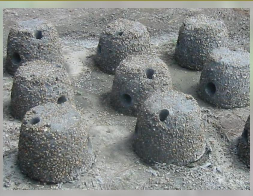
Figure 2: Armored cultivator units post production awaiting deployment. (photo: J. Krumholz)
